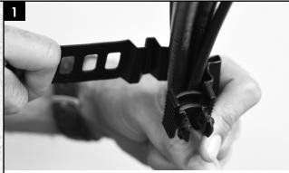
Hold the Snapwrap with the "CABLE BUNDLE THIS SIDE" facing up and place the cables that you want to secure on top of the strap near the edge with the latches.
