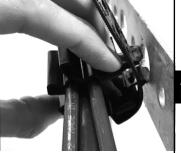
To remove: Press down with thumb and apply pressure with fingers on clip to squeeze latches together and rotate hanger out.
