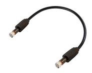
FSJ2-50 SureFlex® Jumper with interface types 4.3-10 Male and 4.3-10 Male with HELIAX® SureGuard weatherproofing, 12 ft
