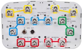
14-port, 1.8m, multiband antenna, RF port assignments are as follows: R1 = 694–862, R2 = 880–960, G1 = 1427–1518, B1 & B2 = 1695–2180 and Y1 & Y2 = 2490–2690 MHz, 65° horizontal beamwidth, 6x Internal RET. Y1 & Y2 share a common RET
