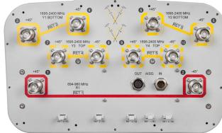
10-port sector/multibeam antenna, 2x 694–960 sector and 8x 1695–2400 multibeam, 65° sector and 33° 4x multibeam, 5x RET with
