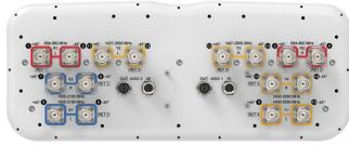
16-port sector antenna, 4x 694–960, 4x 1427–2690, 4x 1695–2180 and 4x 2490–2690 MHz, 65° HPBW, 6x RET
