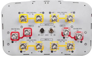
12-port sector antenna, 2x 698–798, 2x 824–896 and 8x 1695–2360 MHz, 65° HPBW, 3x RET and low bands have diplexers
