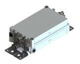
Dual Band Tower Mounted Amplifier, 1800//2100 MHz, 12 dB, 2 BTS & 2 ANT ports, with 4.3-10 connectors, AISG with 1 RET connector (1 device with 2 sub-units each)
