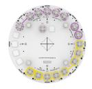
16-port small cell antenna, 8x 1695-2690, 8x 3300-4000 MHz, 360° Horizontal Beamwidth, fixed tilt.
